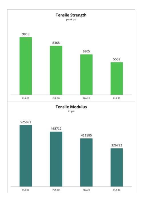
Tensile tests showed that strength and modulus properties declined at a proportional rate to be expected with the incorporation of an elastomer with a rigid polymer. However, elongation properties showed a similar trend to the results of the impact tests. The 10% and 20% samples showed elongation increased by 4.2% and 9.01% respectively. A more dramatic increase of 18.7% in elongation was observed at the 30% sample.
