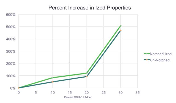
Notched Izod Pendulum Impact tests showed an incremental increase in impact strength at the 10% and 20% levels with greater increases in impact strength achieved between the 20%
