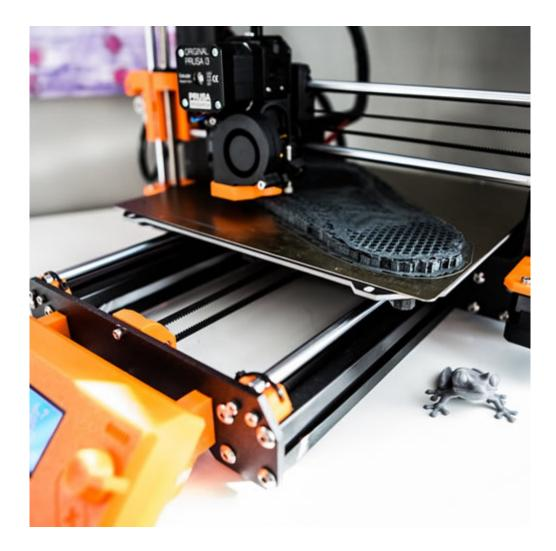
The biodegradable filament used to create the shoes was manufactured by Berlin-based, BioInspirations, using Terratek® Flex, a unique compostable elastomeric bioplastic created by Green Dot Bioplastics. The soft, rubber-like bioplastic is strong and durable, and will biodegrade when placed in an industrial composting environment.
